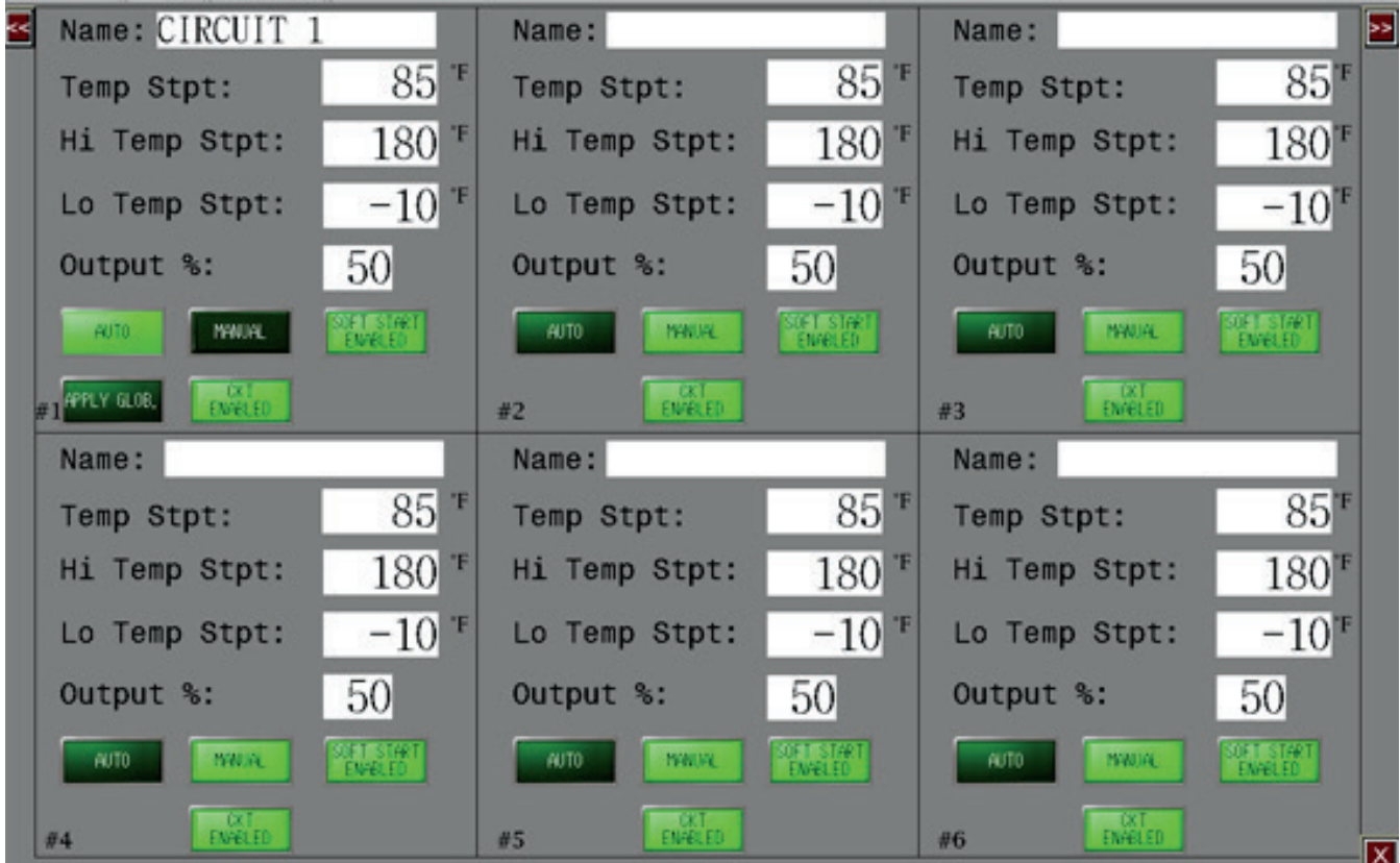
Figure 2A: Freeze Protection/Process Maintain Programming
